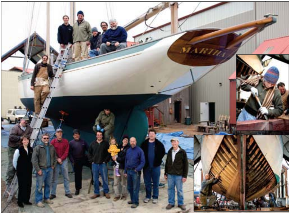
This winter, the 68' schooner Martha underwent a major rebuild at the PT Shipwrights Co-op, located at the Port of Port Townsend Shipyard. Her wooden hull received all new planking and many new frames and timbers. She was re-launched on May 7, attended by scores of well-wishers. Overseeing a largely volunteer labor force were shipwright Antonio Salguero and Martha's captain and caretaker Robert d'Arcy (pictured at center, to the right of his daughter Mary and wife Holly). The 101-year-old vessel is owned and operated by the nonprofit Schooner Martha Foundation ( www.schoonermartha.org ). Photos by Michael Berman
